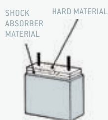
SHOCK ABSORBER AND HARD PLATE (THE TWO PLATES ARE THREADED ON TWO FLEXIBLES AND NOT GLUED)
