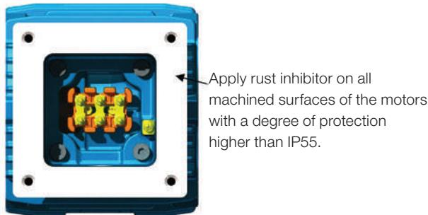
Figure 8.2 - Machined surface of the terminal box of explosion-proof Motors.
