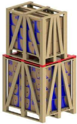
Figure 5.5 – Use of additional battens for stacking
