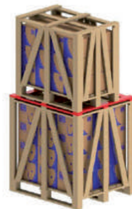
Figure 5.5 - Use of additional battens for stacking
