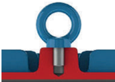
Figure 4.1 - Correct tightening of the eyebolt
