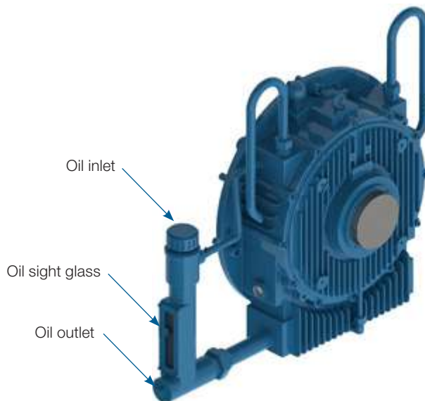
Figure 8.2 - Oil lubricated bearing - horizontal mounting
