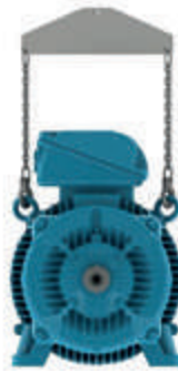
Figure 4.7 - Use of a spreader beam for lifting
