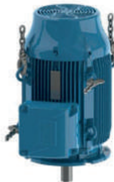
Figure 4.18 - Install the second pair of eyebolts
