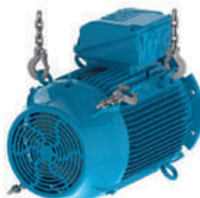
Figure 4.11 - Installation of the second pair of eyebolts
