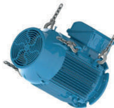
Figure 4.19 - Motor is being rotated to horizontal position
