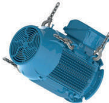
Figure 4.19 - Motor is being rotated to horizontal position
