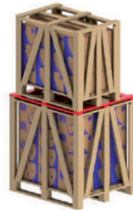
Figure 5.5 - Use of additional battens for stacking
