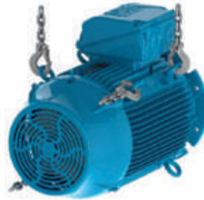
Figure 4.11 - Installation of the second pair of eyebolts
