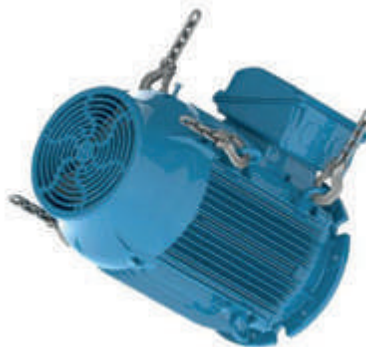
Figure 4.19 - Motor is being rotated to horizontal position
