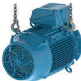
Figure 4.10 - Removing the motor from the packaging
