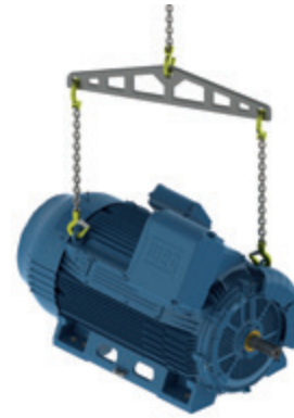
Figure 7 - Lifting with vertical chains.
