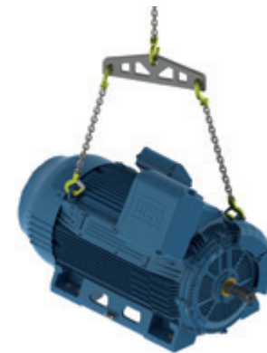
Figure 8 - Lifting with inclined chains.
