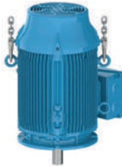
Figure 4.17 - Install the first pair of eyebolts
