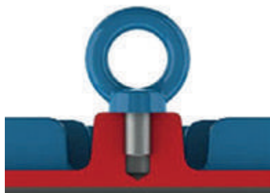
Figure 4.1 - Correct tightening of the eyeboll
