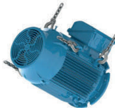
Figure 4.19 - Motor is being rotated to horizontal position
